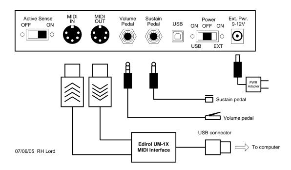
The "Active Sense" switch implements a feature of MIDI that can detect if the MIDI connection stops working. When "Active Sense" is on, the Lambdoma keyboard will repeatedly send the "Active Sense" MIDI message in the absence of any other keyboard output. If your MIDI device gets confused by this message, switch it off.
